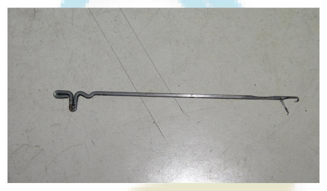
Loops are formed during the process of knitting by raising and lowering needles. As the needle raises, old yarn loop opens the latch and as the needle reaches the maximum height, it receives new yarn. The needle then starts descending down hence, the old loop knocks over and the new loop is held in the needle.
